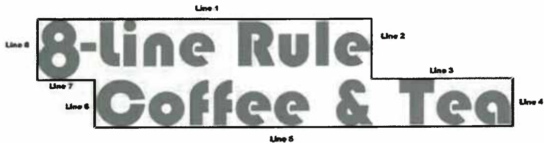
Figure 7100.2: Measuring Building-Mounted Sign Area
