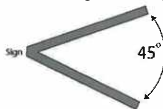
Figure 7100.3: Measuring Multi-faced Sign Angle
