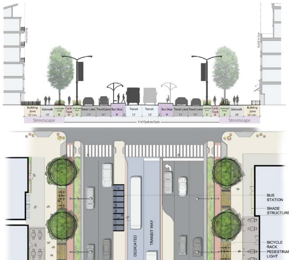
Figure 35 – Transit Boulevard Median Running Cross-section
