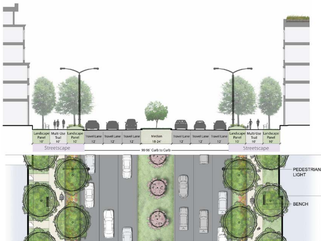
Figure 34 – Multimodal Through Corridor Cross-section
