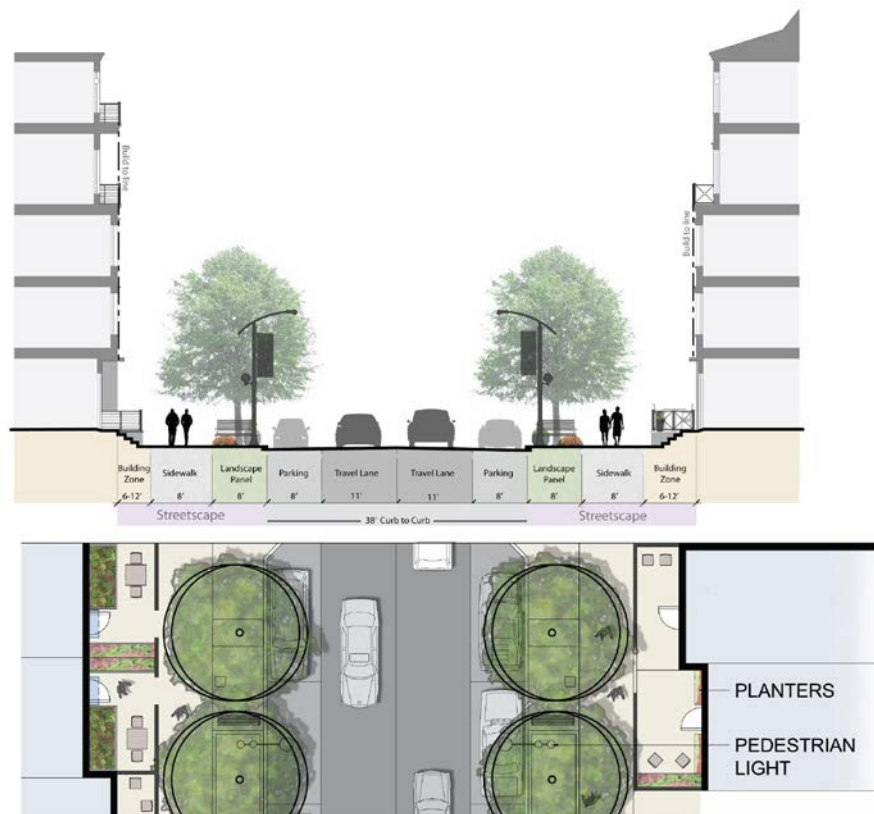
Figure 38 – Local Street Cross-section
