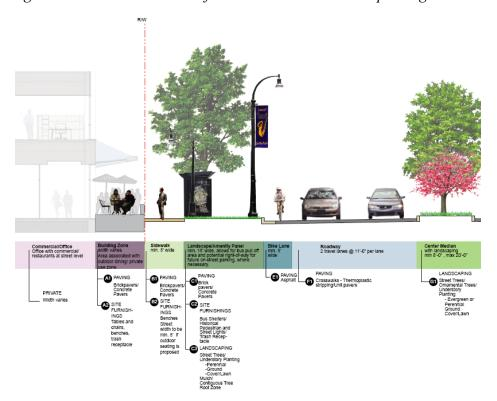
Figure 16: Typical Intersection Improvement Plan- Minor Arterial to Minor Arterial
