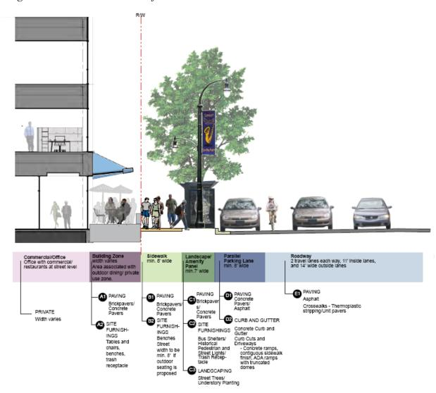
Figure 19: Typical Intersection Improvement Plan- Collector Street to Minor Arterial
