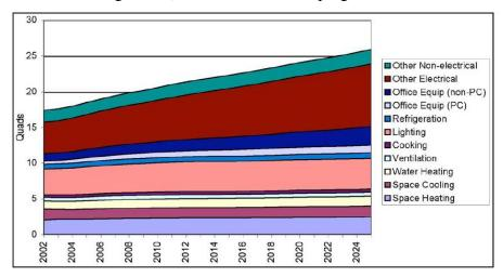
Figure 4: Commercial building energy consumption by use (ORNL, 2004)
