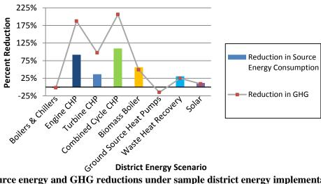
Figure 6: Source energy and GHG reductions under sample district energy implementations (built from FVB, 2011)
