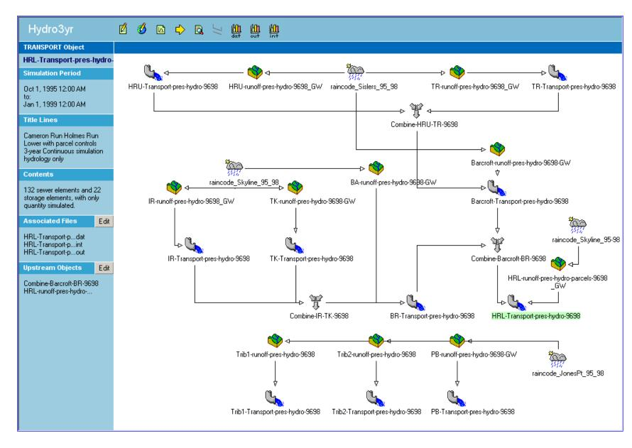
Figure 2-1. Cameron Run watershed SWMM model components as shown in the PCSWMM Object Manager
